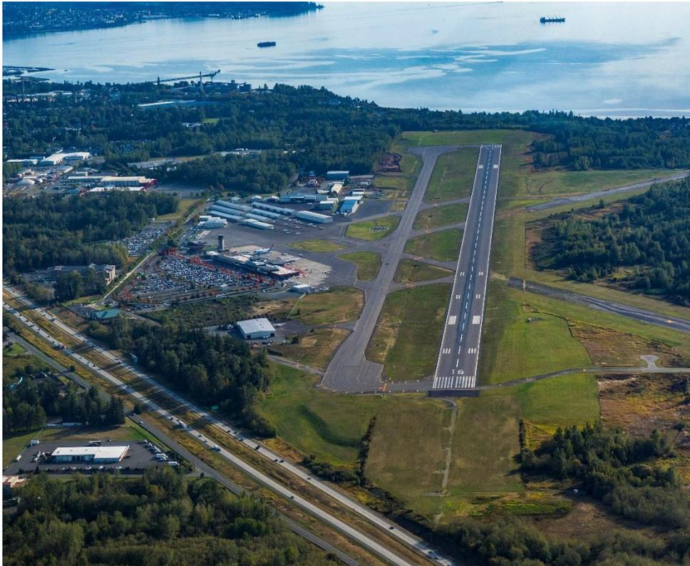
BLI is an FAA Class 1, Part 139 airport, located on 1,018 acres just north and west of the City of Bellingham. It's equipped with a 6,701 x 150-foot all-weather precision Instrument Landing System (ILS) Runway 16-34 controlled by an FAA contract Air Traffic Control Tower. There are visual approach landing aids to both the 16 and 34 runway approaches.
