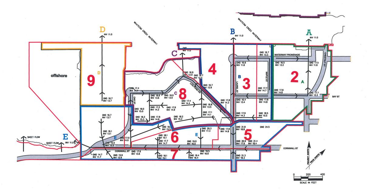
GND XX.X FUTURE GROUND ELEVATION INV XX.X PIPE INVERT ELEVATION BASED ON PIPES AT 0.3% SLOPE
