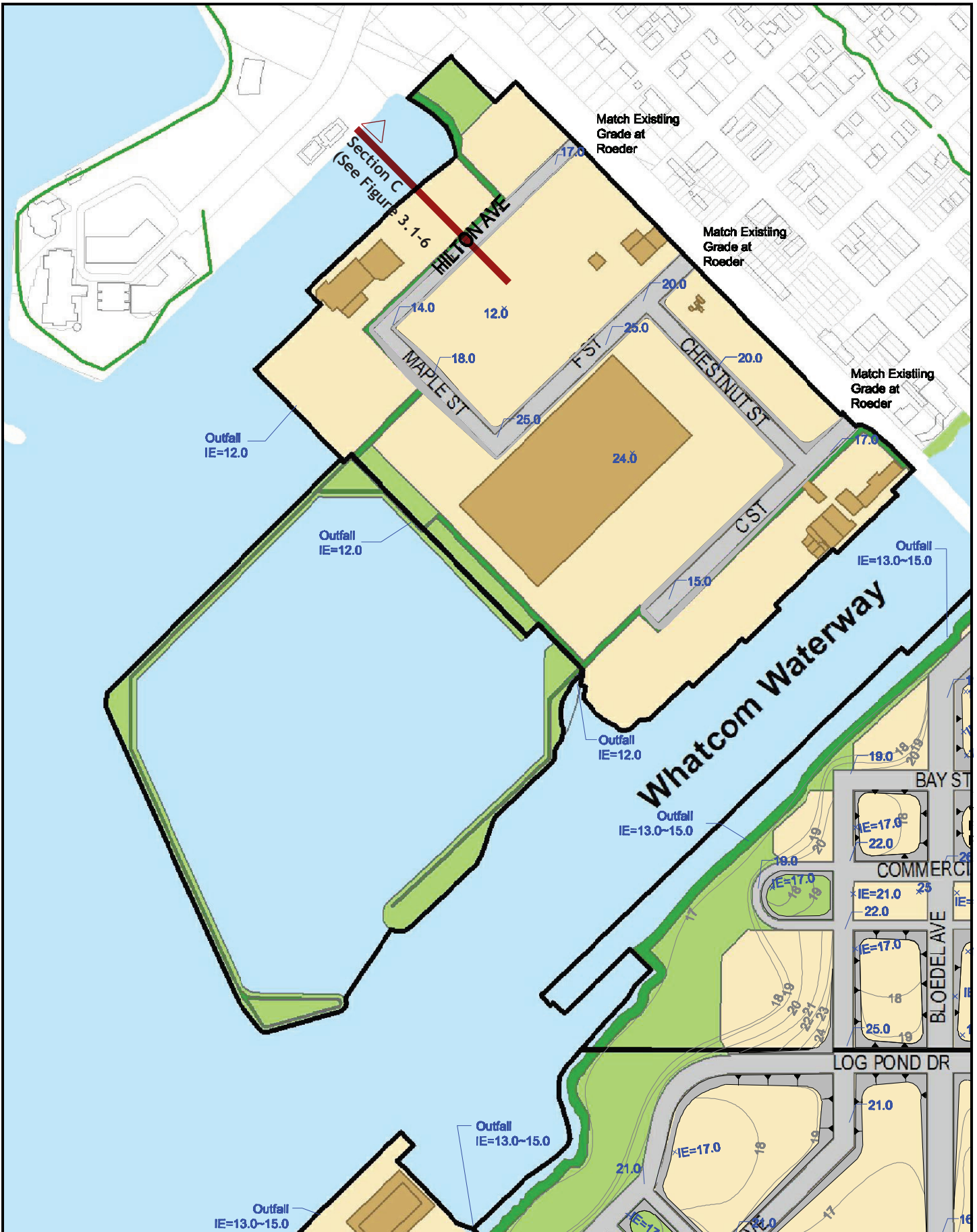
Figure 3.1-1 Marine Trades Area Grading Plan Preferred Alternative
