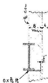
TYPICAL SPANDREL DETAIL
